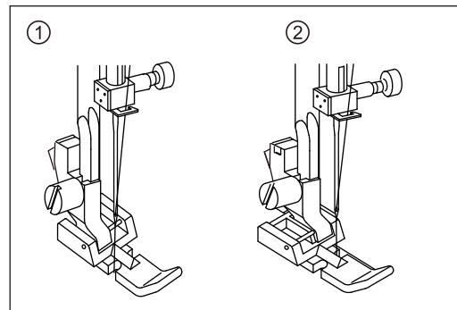
Align the right side or the left side of the zipper foot pin with the presser foot holder, lower the presser foot lever to attach the foot.
