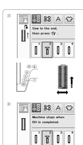
3 Start sewing again, and the machine sews the front bartack and right side of the buttonhole. Stop the machine when you reach the ending point. Then press the reverse button ①.
