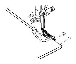
Attach 1/4" seam foot O (optional item), which helps you to keep a constant 1/4" (6 mm) seam allowance. Put 2 pieces of fabric with right sides together. Place the patchwork pieces under the foot so that the edge of the fabric matches the guide on the presser foot.
